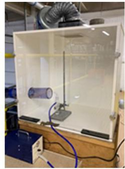
SKC Air Sampler inside chamber
