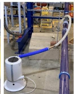
Cyclone Sampler on horizontal drain
