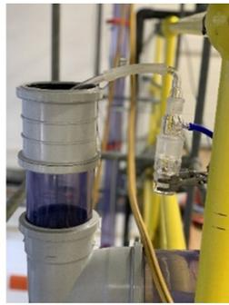
SKC Air Sampler at stack top
