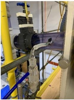
SKC Air Sampler chamber branch drain
