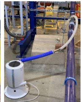
Cyclone Sampler on horizontal drain
