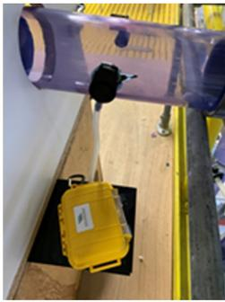
SolidSense sampler on chamber branch
