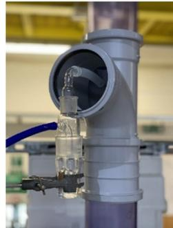
SKC Air Sampler at test-point on stack
