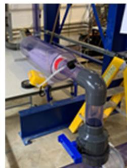
Containment bag in cylinder on horizontal drain
