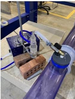
SKC Air Sampler on horizontal drain (closed pipe)
