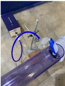
SKC Air Sampler on horizontal drain (open pipe)
