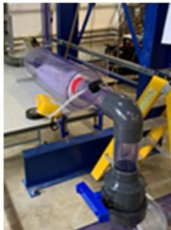
Containment bag in cylinder on horizontal drain
