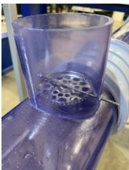
Passive air sampler on horizontal drain
