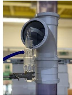
SKC Air Sampler at test-point on stack
