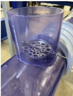
Passive air sampler on horizontal drain
