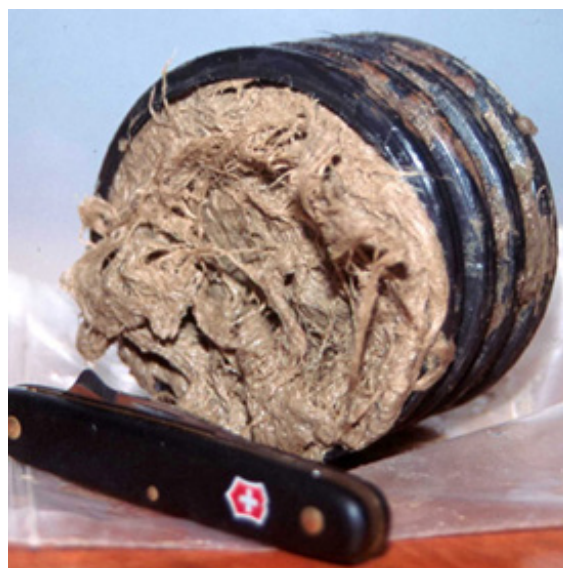
Figure A1:1 – Agricultural drains can be blocked by a mix of roots and soil. Source: Leuty (2012).
