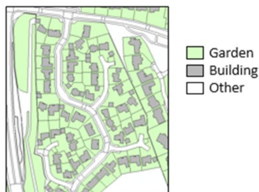
Figure 11 Identify garden polygons from OS data (buildings and roads are already identified in the data).
