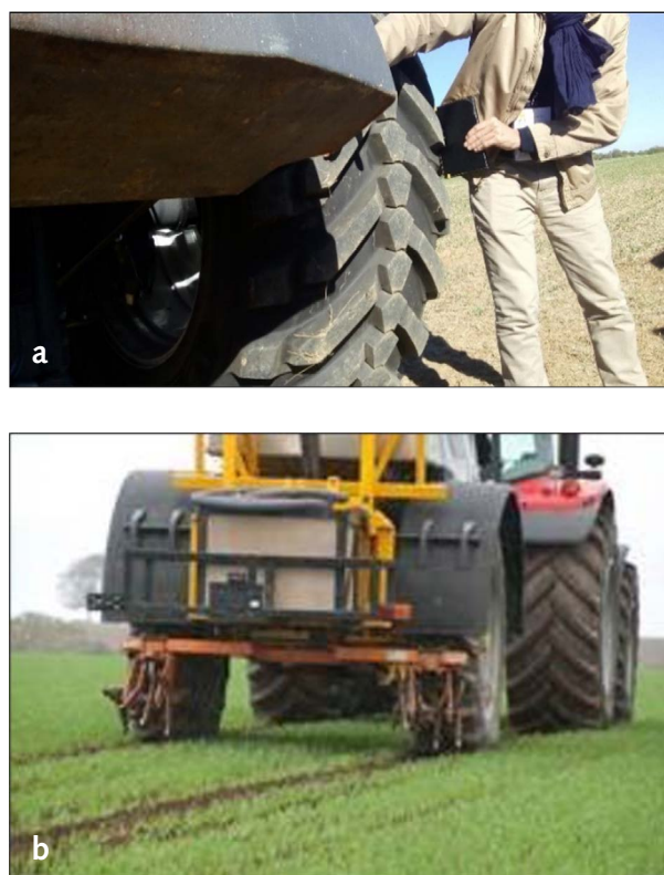
Figure 4. Photographs of a) the new EVOBIB and b) the older XEOBIB tyres. Note the block shapes in the centre of the tread in the new EVOBIB tyre and the spiked harrow used alongside the XEOBIB tyre for loosening the soil (courtesy of B. McKenzie).
