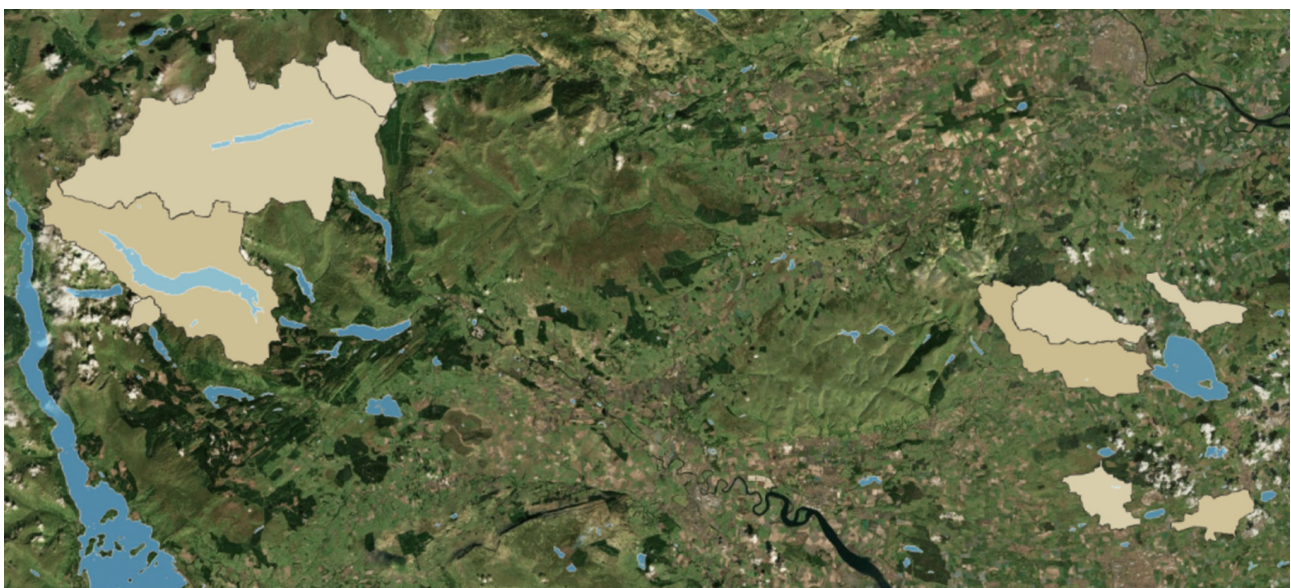
Figure 2 Example of sub-catchments generated using SEPA inflow monitoring station locations.
