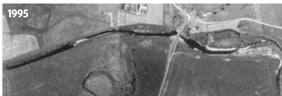
The upper River Spey at Laggan, 5 km downstream of Spey Dam in 1946 (four years after dam construction) and in 1995. Narrowing of the channel and stabilisation of previously active gravel bars are linked to a history of upstream flow regulation and straightening (© Centre for River Ecosystem Science).
