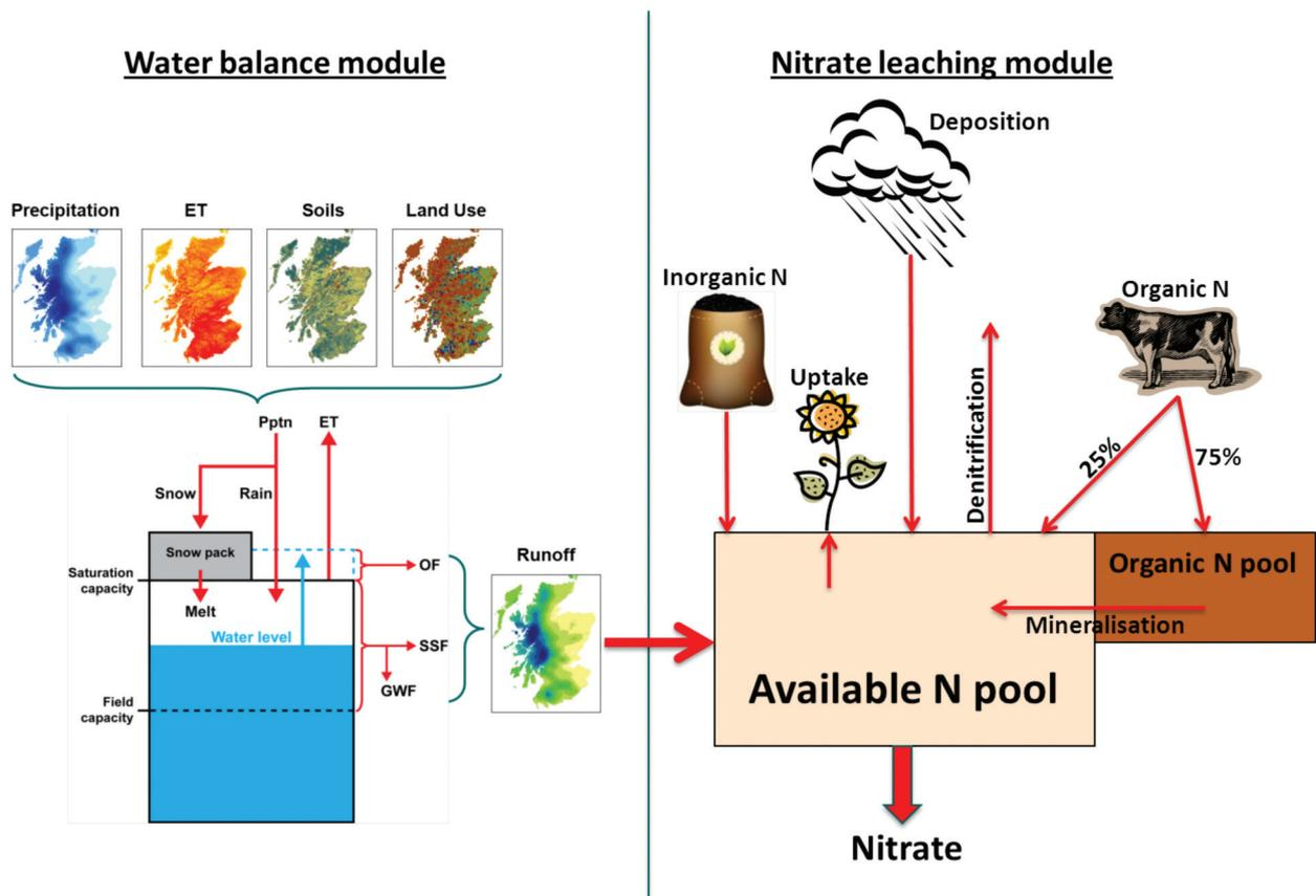
Fig. 5: Illustration of the NIRAMS II model structure, showing key input datasets and physical processes. OF, overland flow; SSF, shallow sub-surface flow; GWF, groundwater flow.
