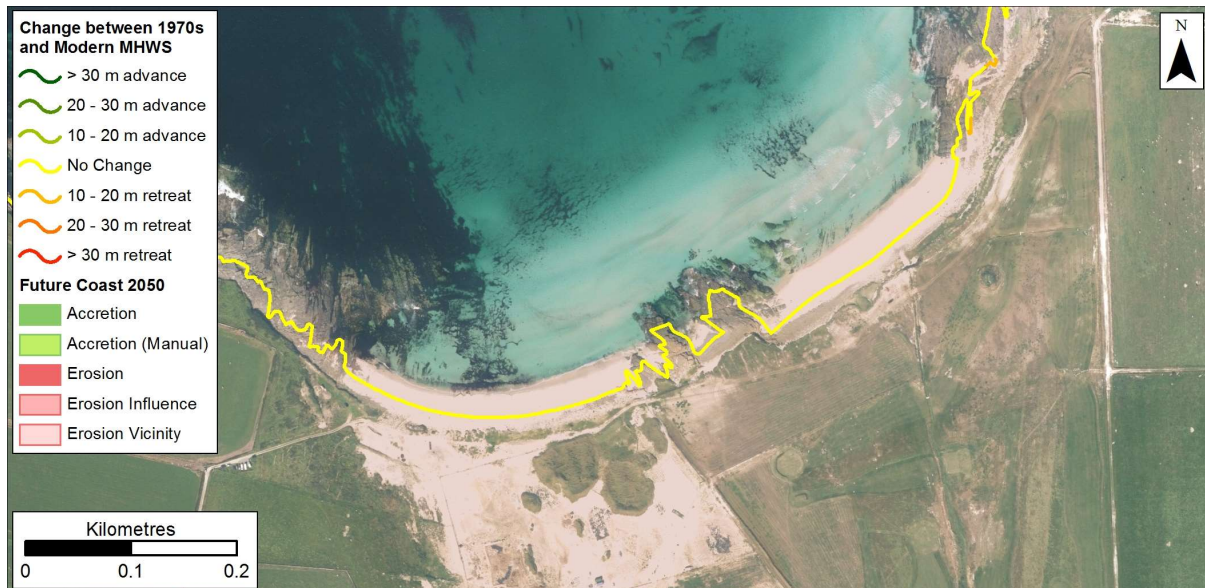
Figure 10.30: Possible future coastline position in 2050 based on rates between 1970 and Modern MHWS data at the Links of Notland. Getmapping are our current providers of Scotland-wide digital aerial imagery© Getmapping plc.
