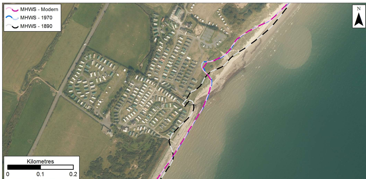
Figure 7.3: MHWS position in 1890, 1970s, and Modern datasets at Sandhead, Luce Sands. Getmapping are our current providers of Scotland-wide digital aerial imagery© Getmapping plc.
