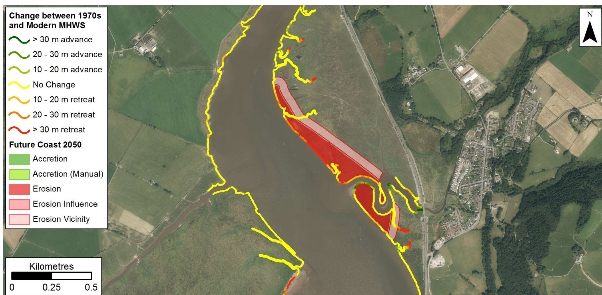
Figure 7.9: Possible future coastline position in 2050 based on rates between 1970 and Modern MHWS data Creetown. Getmapping are our current providers of Scotland-wide digital aerial imagery © Getmapping plc.
