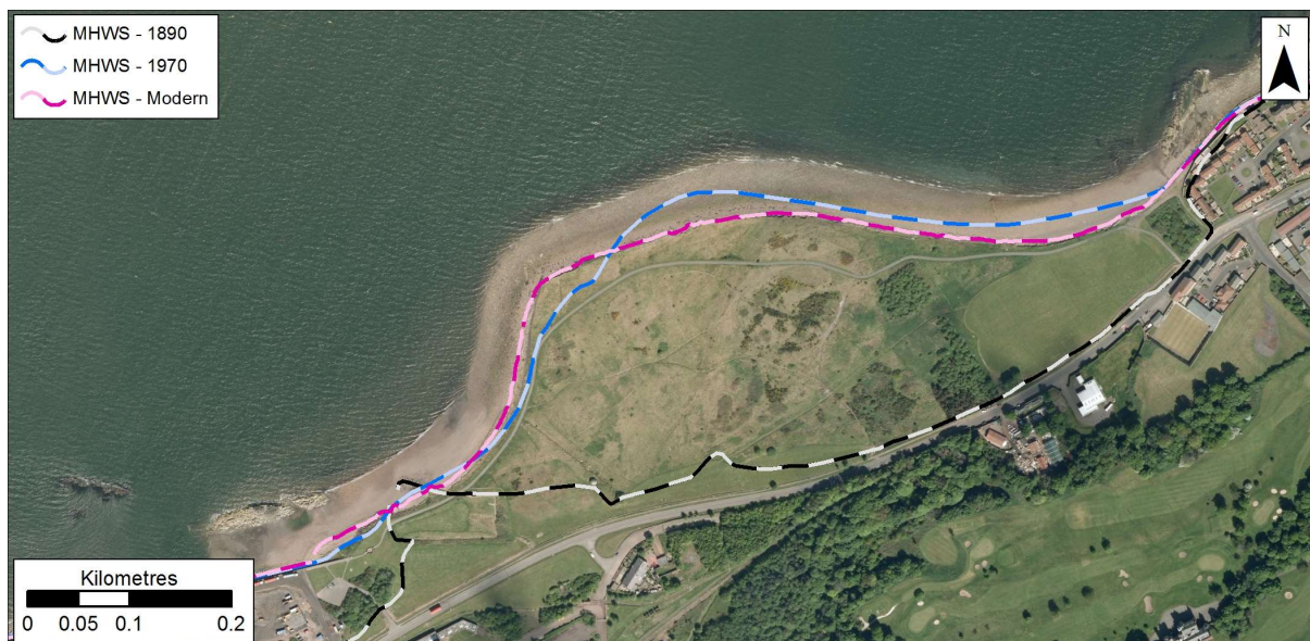
Figure 1.16: MHWS position in 1890, 1970s, and Modern datasets at east of Prestonpans. Getmapping are our current providers of Scotland-wide digital aerial imagery© Getmapping plc.
