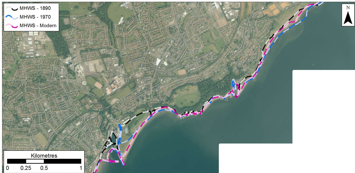
Figure 1.23: MHWs position in 1890, 1970s, and Modern datasets at Dysart. Getmapping are our current providers of Scotland-wide digital aerial imagery© Getmapping plc.
