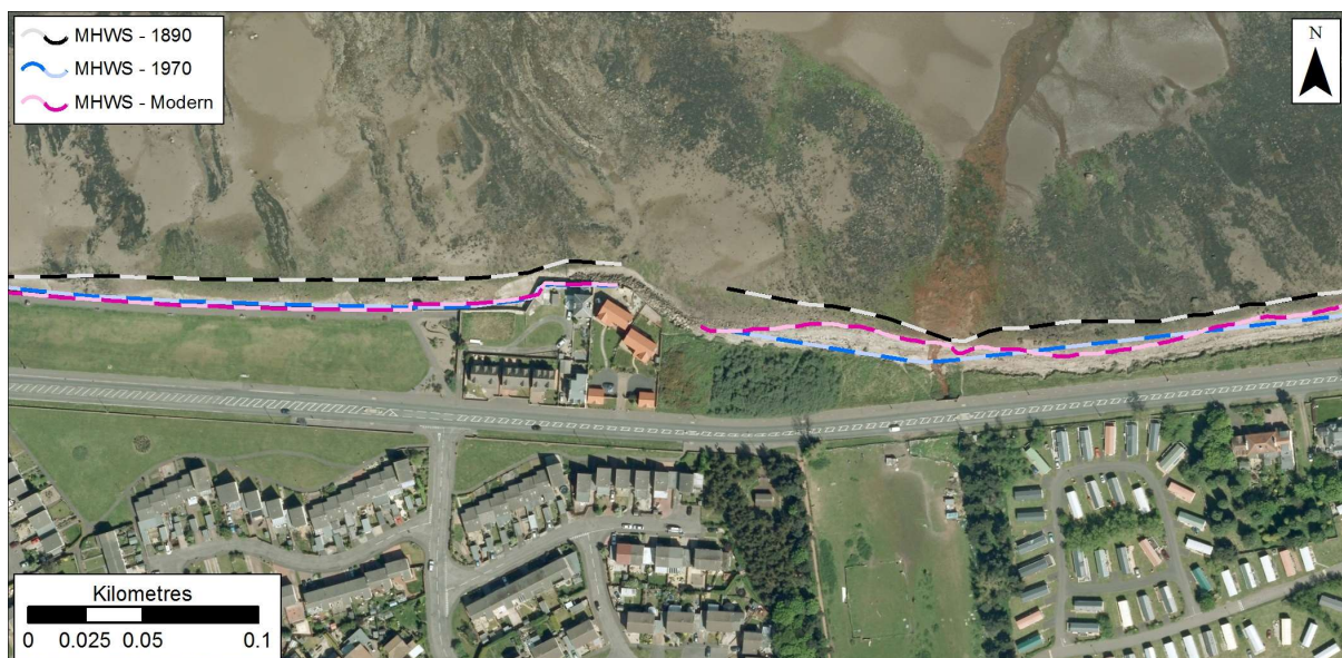
Figure 1.12: MHWS position in 1890, 1970s, and Modern datasets at Port Seton. Getmapping are our current providers of Scotland-wide digital aerial imagery© Getmapping plc.
