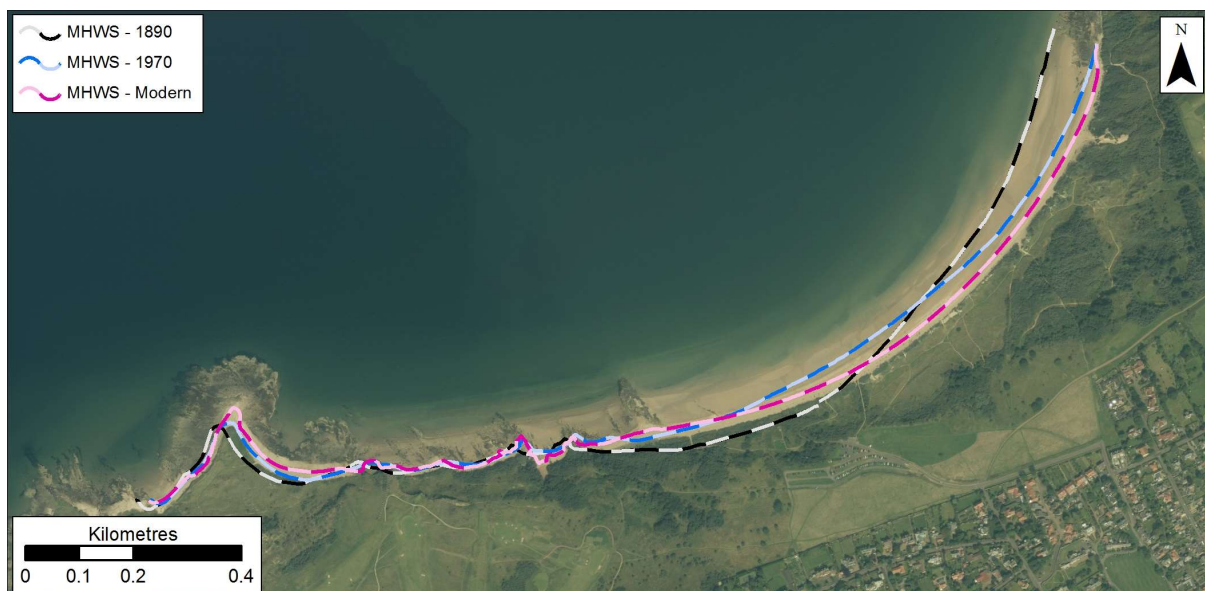
Figure 1.10: MHW position in 1890, 1970s, and Modern datasets at Gullane Bay. Getmapping are our current providers of Scotland-wide digital aerial imagery© Getmapping plc.
