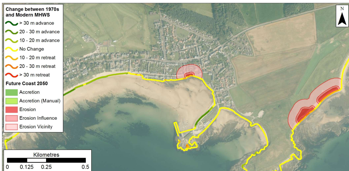
Figure 1.31: Possible future coastline position in 2050 based on rates between 1970 and Modern MHWs data at Earlsferry. Getmapping are our current providers of Scotland-wide digital aerial imagery© Getmapping plc.
