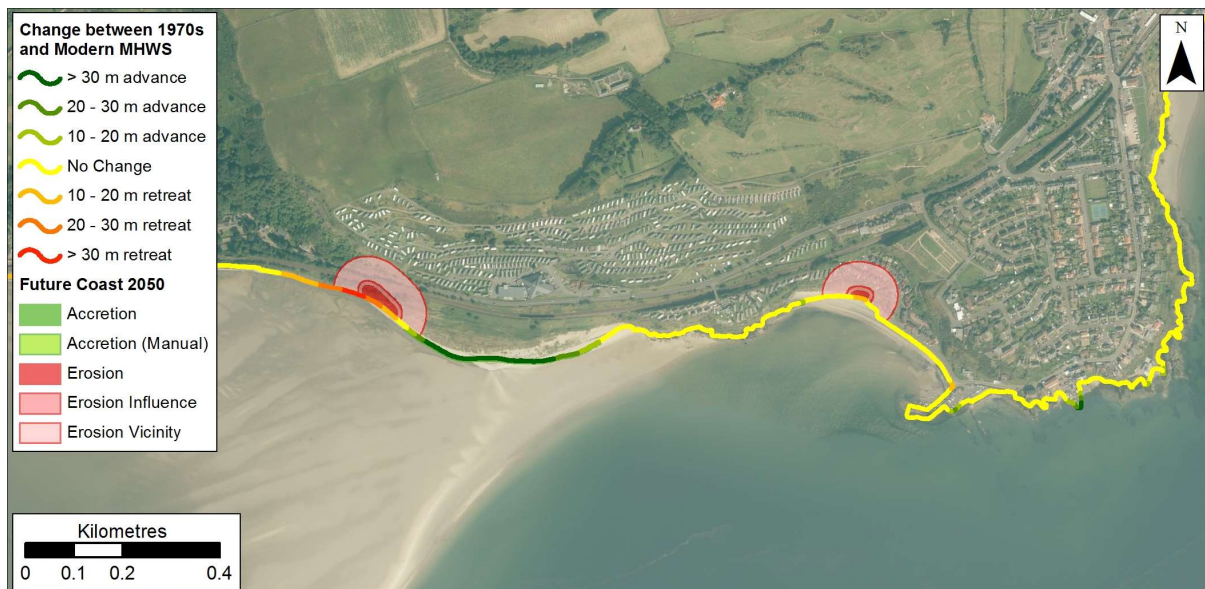
Figure 1.22: Possible future coastline position in 2050 based on rates between 1970 and Modern MHW data at Kinghorn. Getmapping are our current providers of Scotland-wide digital aerial imagery© Getmapping plc.
