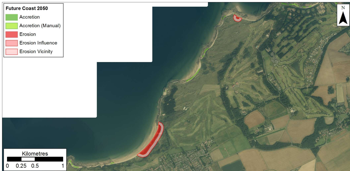
Figure 1.11: Possible future coastline position in 2050 based on rates between 1970 and Modern MHWS data at Gullane Bay. Getmapping are our current providers of Scotland-wide digital aerial imagery© Getmapping plc.
