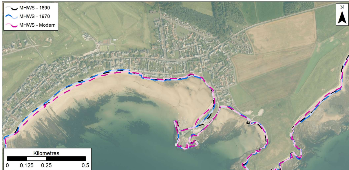
Figure 1.30: MHWs position in 1890, 1970s, and Modern datasets at Earlsferry. Getmapping are our current providers of Scotland-wide digital aerial imagery© Getmapping plc.
