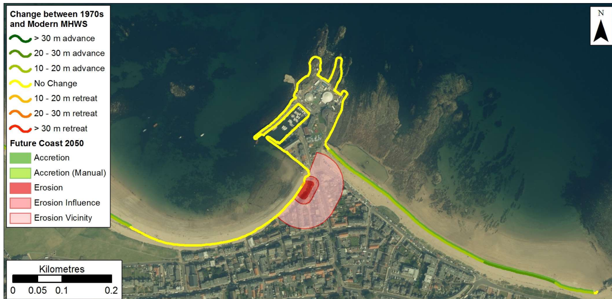
Figure 1.9: Possible future coastline position in 2050 based on rates between 1970 and Modern MHWS data at North Berwick. Getmapping are our current providers of Scotland-wide digital aerial imagery© Getmapping plc.
