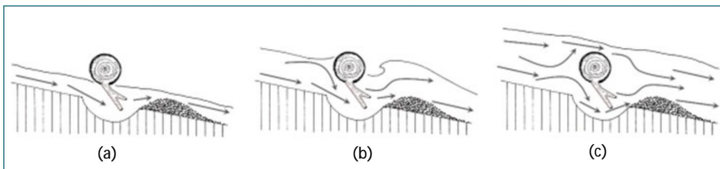
Figure 2.8: Cross-section view of Category B type placements showing the changes in flow conditions under (a) less than bankfull river levels, (b) over bankfull levels and, (c) very high river levels.
