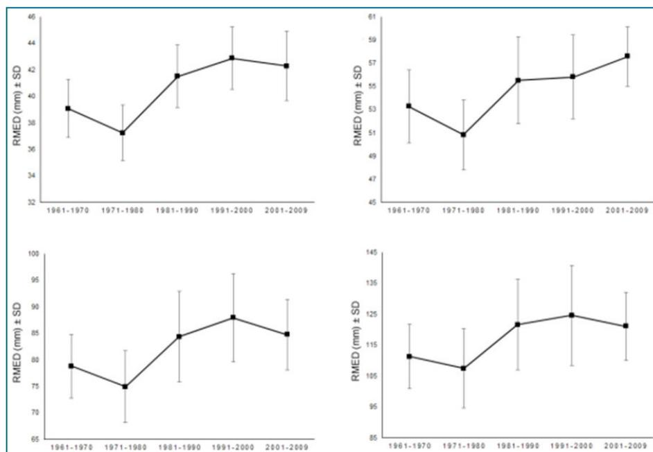
Figure 1.1: Increasing trends in the intensity of rainfall in Scotland (measured as RMED; RMED is defined as the median of annual maximum rainfalls (for a given duration) at a site) for (a) 1 day, (b) 2 day, (c) 5 day and, (d) 10 day durations from 1961 to 2009. Data adapted from Table 2 in Jones et al. (2013).
