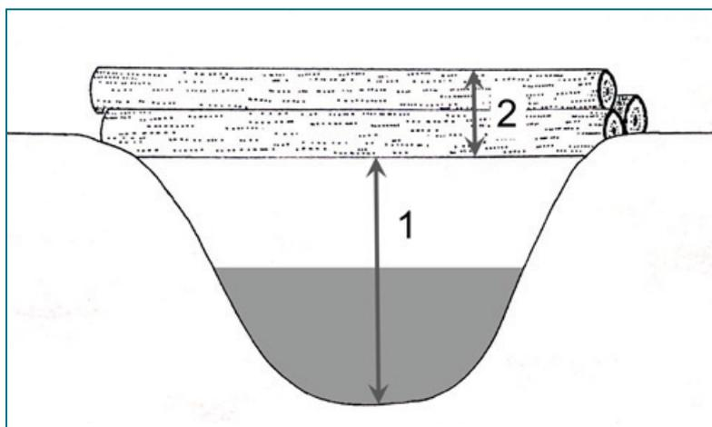
**Figure 6.1:** In-river view schematic of Category A type placements detailing the two physical attributes to be considered with respect to the fish fauna present at a site (1) the minimum distance between the bed of the river and the bottom of the woody placement and, (2) the vertical height of the placement
