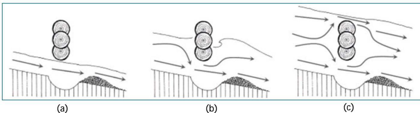
Figure 2.7: Cross-section view of Category A type placements showing the changes in flow conditions under (a) less than bankfull river levels, (b) over bankfull levels and, (c) very high river levels.
