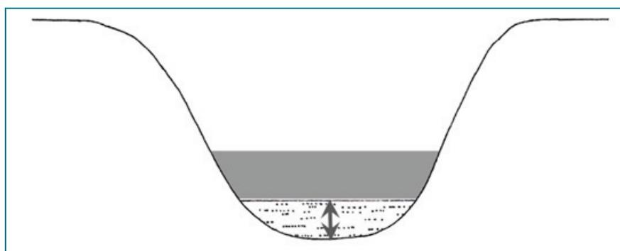
**Figure 6.5** The height of the timber, measured from the river bed to the top of the timber is the key physical characteristics of this woody placement type
