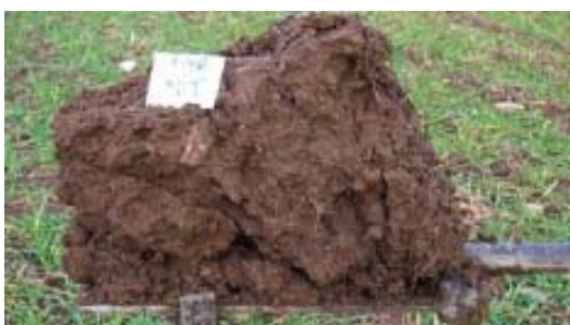
Visual assays will quickly assess compaction damage and drainage issues. A subset of farms will have detailed monitoring.
